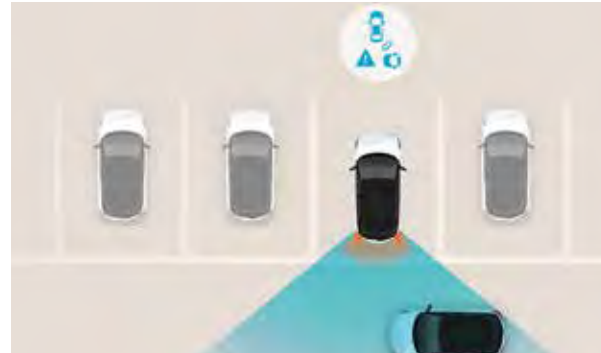
Rear Cross-Traffic Collision-Avoidance Assist (RCCA): Perfect for car parks. When reversing out of areas with low visibility, the system not only warns the driver if vehicles approach from the side, it also applies the brakes automatically.
